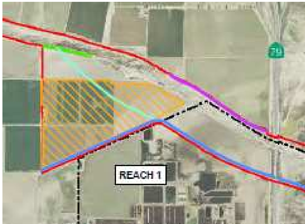
Figure 13-1 – Conceptual footprint of in-channel sedimentation basin located at the downstream reach of the levee system
