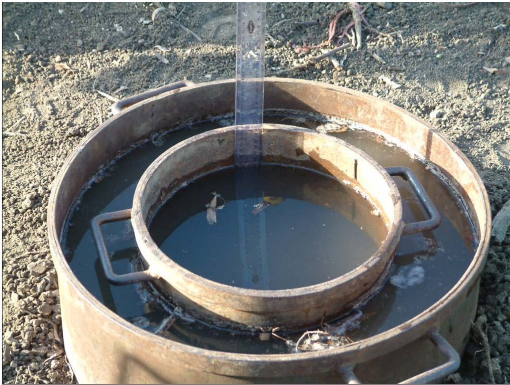
Photo 2 – Simple Double Ring Infiltrometer
