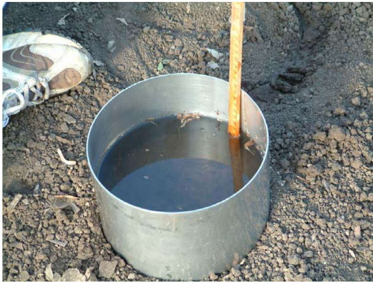
Photo 1 – Simple Single Ring Infiltrometer
