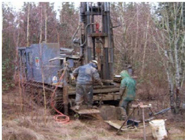
Photo 8- Auger Boring Rig
