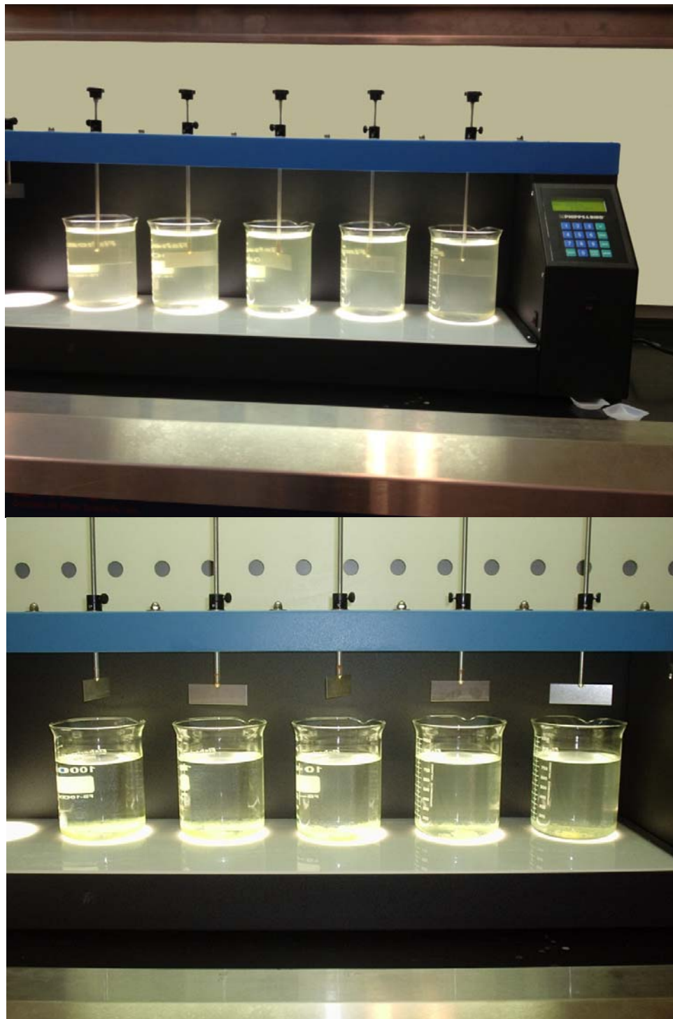
Figure 1. Phipps and Byrd jar testing apparatus used in this study, at the beginning (top) and at the end of the test procedure after settling of the flocs (bottom).
