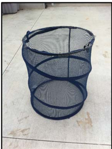
Figure 5. Collapsible hamper, used to quantitatively collect all water column macroalgae within a designated surface area and volume of water column
