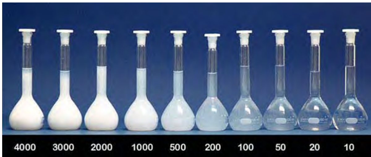
Figure 1. Comparison turbidity from 10 NTU to 4000 NTU. ( http://www.optek.com/Turbidity_Measurement_Units.asp )
