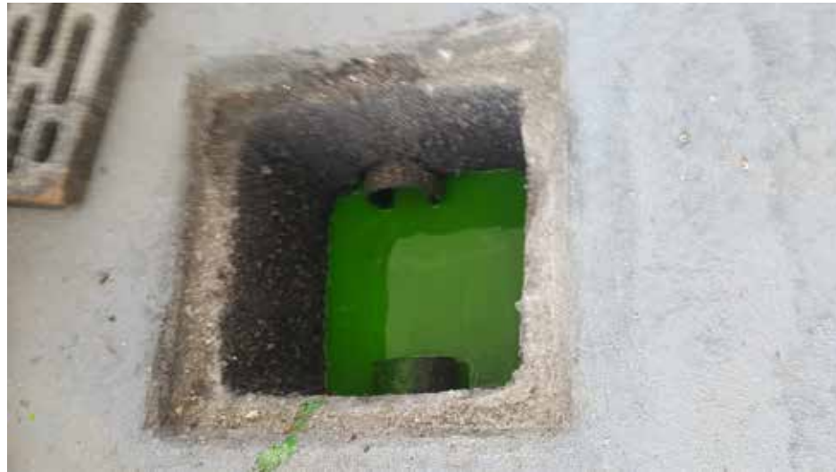
Tracer Dye Added to Sump near outdoor conveyor system
