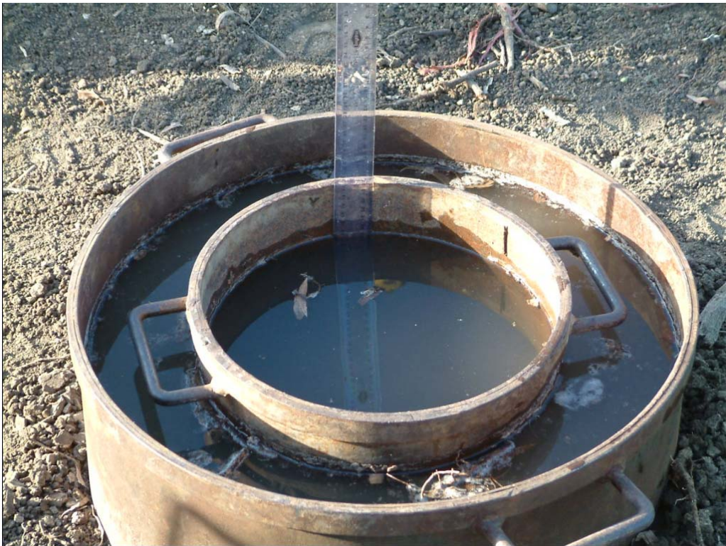
Photo 2 – Simple Double Ring Infiltrometer
