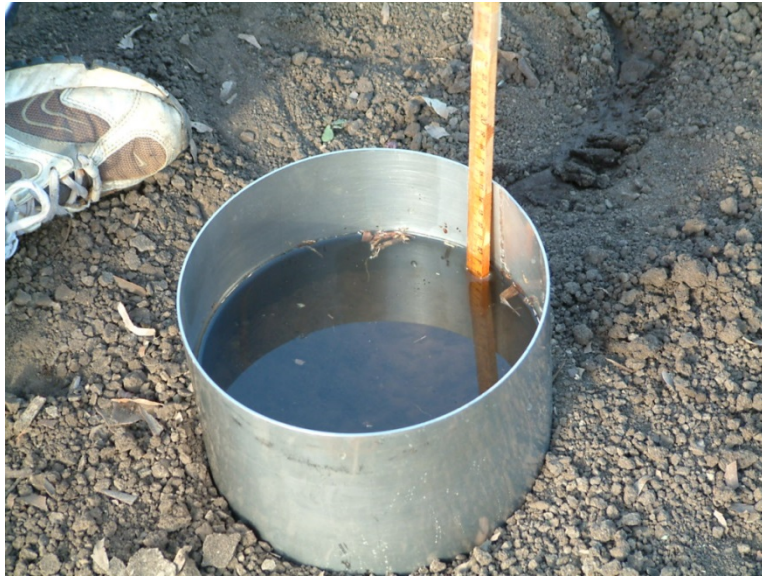
Photo 1 – Simple Single Ring Infiltrometer
