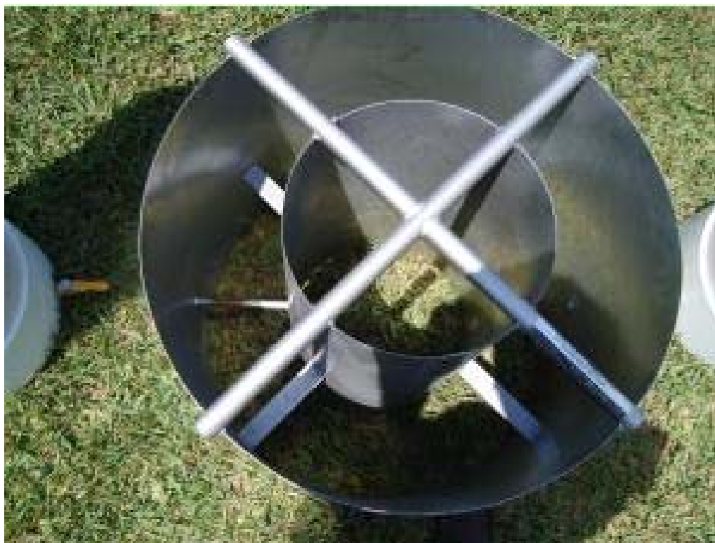
Photo 3 – Pre-fabricated Double Ring Infiltrometer (Photo courtesy of Turf-Tec International)
