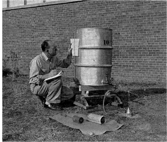
Photo 7 - Typical Well Permeameter Test Installation
