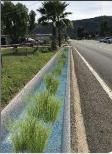
Figure 2-3. Example Rendered Subsurface Wetland Channel During Wet Weather
